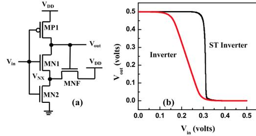
Fig. 1. (a) Basic ST inverter used in [3]. (b) Characteristics of inverter and ST inverter for  $0 \rightarrow 1$  transition at the input ( $V_{dd}=0.5$  V).
