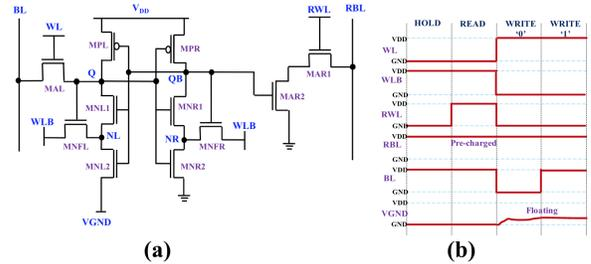
Fig. 2. (a) Schematic and (b) timing of the control signals for the ST11T SRAM cell proposed in [3].
