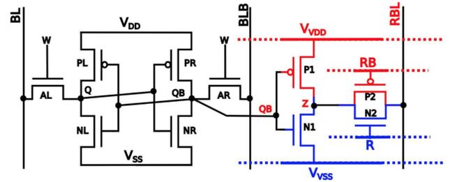
Fig. 3. 10T SRAM cell with row-wise read port dynamic power lines.
