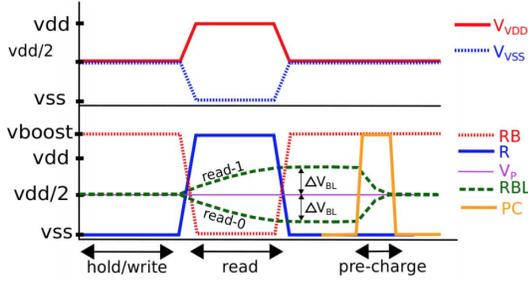
Fig. 4. Levels of control signals during read and otherwise.
